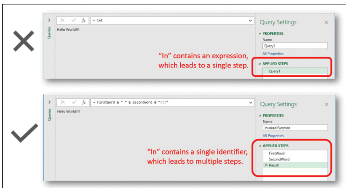
FIGURE 9-4 Having an expression instead of an identifier after the in section in the Advanced Editor leads to a single step in Applied Steps. The preceding M statement demonstrates the solution.
