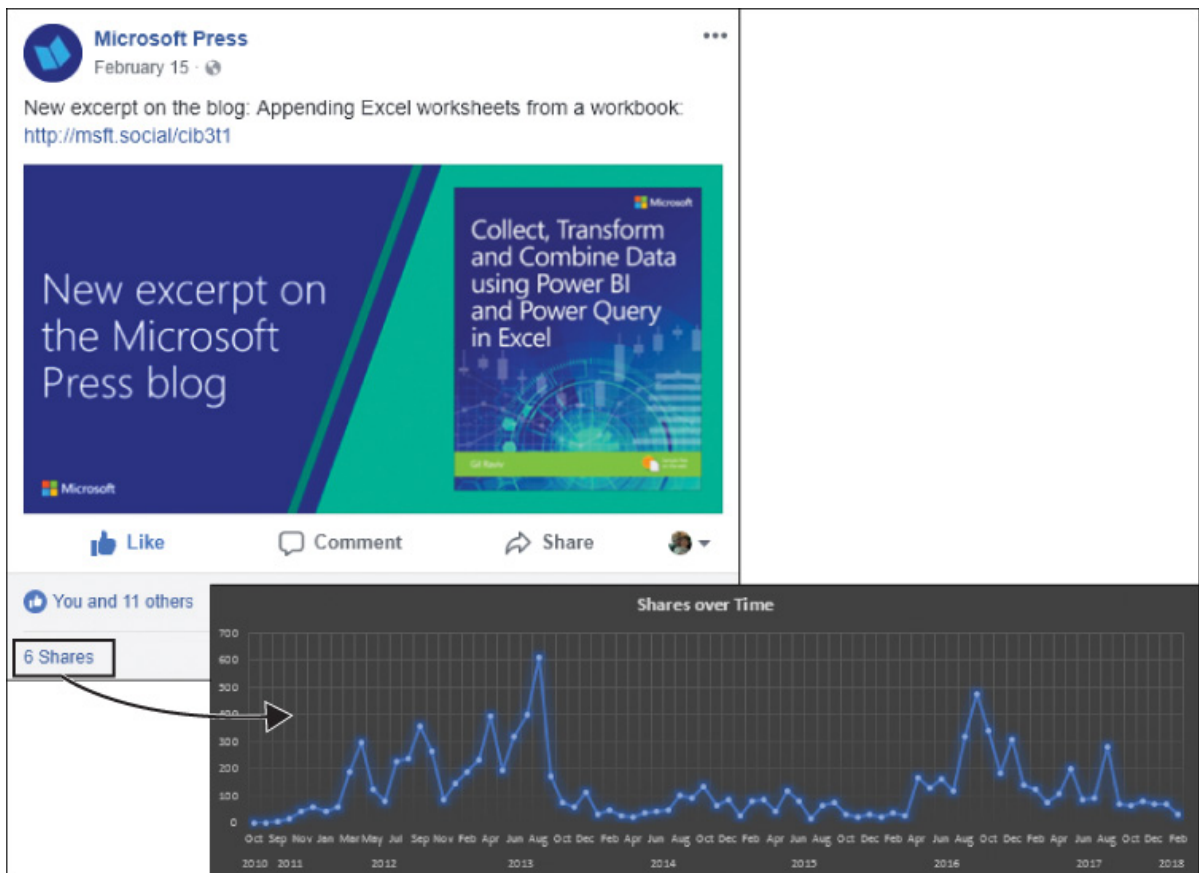
FIGURE 13-8 The Facebook connector enables you to measure user engagement by extracting the number of shares for each post.
